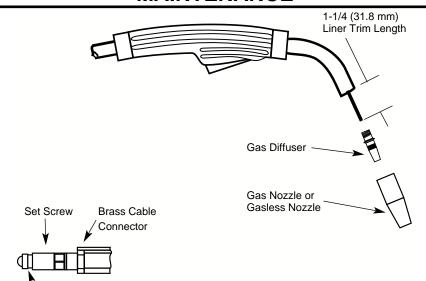
(Liner bushing to be sealed tight against brass cable connector)
